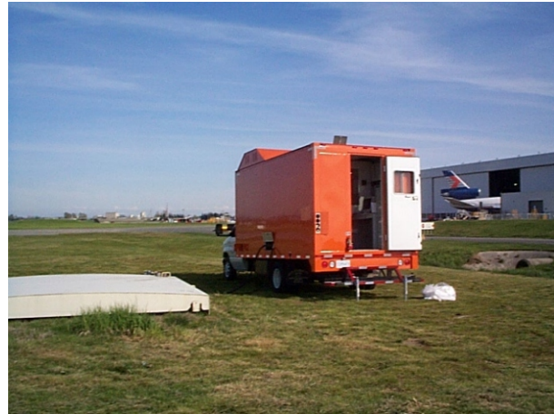
The HT-100 can be permanently installed on a line (or multiple lines), or it can be mounted in a truck or trailer in order to test lines at different locations.
