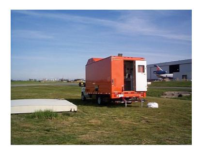
The mobile HT-100 can be transported to distant lines for periodic testing. In some cases it is used by different facilities, which apportion costs commensurate with usage.
