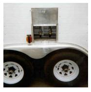
The HT-100 is connected to the pipeline through an opening in the side of the truck/trailer.
